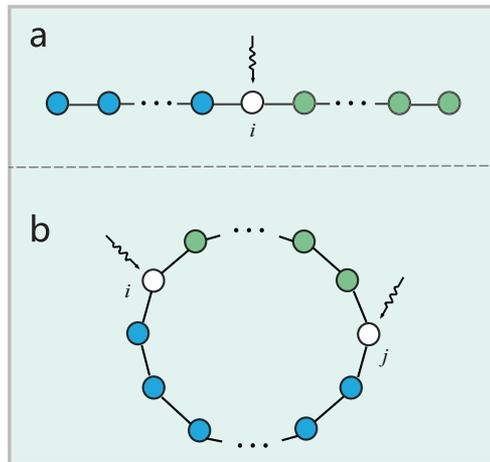
Fig. 1: (Color online) Illustration of network models and construction in this letter. (a) Chain graph with an external control input imposed on node  $i$ , represented as a wavy arrow. (b) Ring graph with node  $i$  and node  $j$  are both controlled. When  $i = j$ , the control inputs degenerate to one controller.
